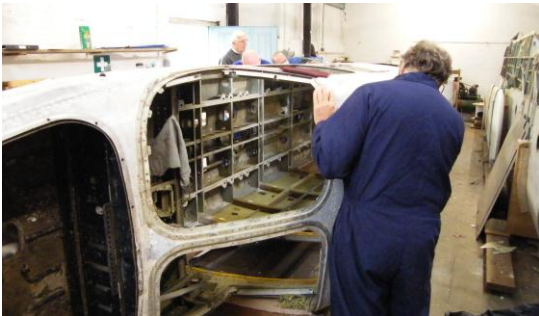
De-corroding in progress
