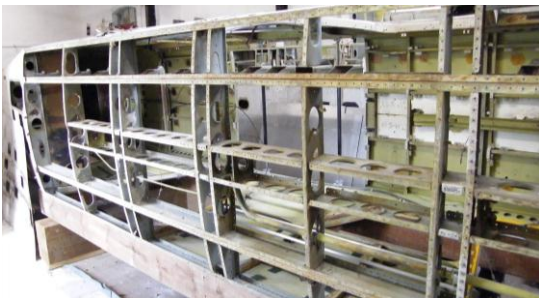
View of under-floor frame structure
